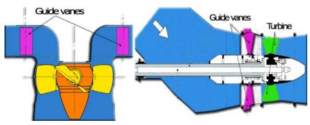
The axial velocity is given by the speed / throughput section. In our example we will assume that the pass section of the guide vanes is equal to the section swept by the turbine blades( $2.01m^2$  for our example), but this is not always the case, as it can be useful to have a low speed in the guide vanes to minimize losses, and deflection angles of fins.
