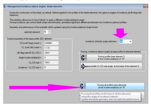
Our stator is rebuilt with profiles whose incidence is forced to 16 degrees. **2 Results hold our attention**:
