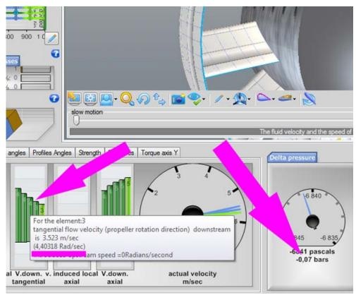
The **tangential velocity** produced is about **4 rad/sec** and the pressure loss is **0.07 bars about 0.7 meters.** We finished the calculation of our stator guide vanes ring type,,
