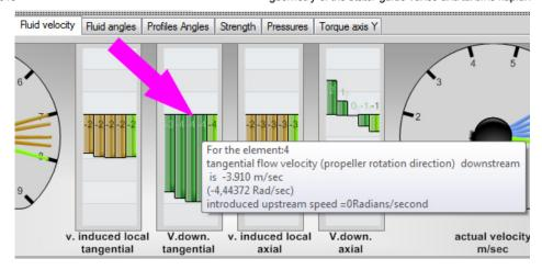
In our example, the induced tangential velocity downstream of the turbine is around **4.4 rad/sec** at the element level **4.So we need to introduce a tangential velocity of 4.4 rad / sec with our stator guide vanes.** For this, use the parameter menu / introduce a tangential velocity, and enter **4.4** rad / sec:
