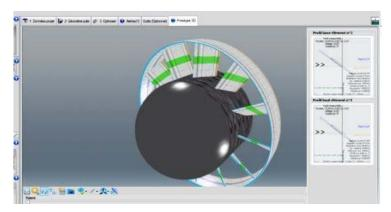
A **ring-type guide vanes is a propeller does not rotate (stator**). We will use Heliciel to calculate the delta pressure between the upstream and downstream of a propeller with a speed of almost zero rotation, and a number of blade, corresponding to the number of blades in our guide vanes. The propeller should generate a tangential velocity downstream of about 4.4 rad / sec. We can even, if we wish, export the 3D igs file stator blades, to a CAD to realize them.
