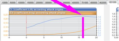
and deduce that the **angle of attack**, **generating most Cz** (lift) thus the more tangential force , is 16 degrees to the naca 6412 at Re 1 million. So we **force angle of attack** to 16 degrees using the "parameter menu / manage forcin angle incidences:
